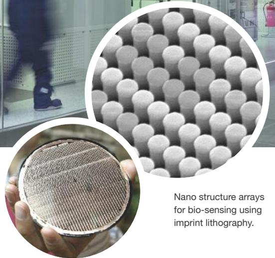
Nano structure arrays for bio-sensing using imprint lithography.
