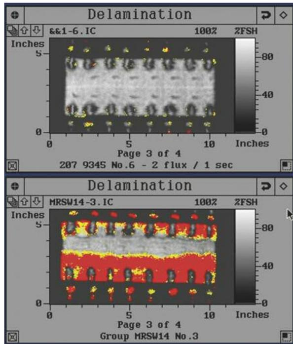
Acoustic images of two plastic packaged integrated circuits. The lower image shows large areas of delamination where the plastic encapsulant has detached from the lead-frame/die paddle.
