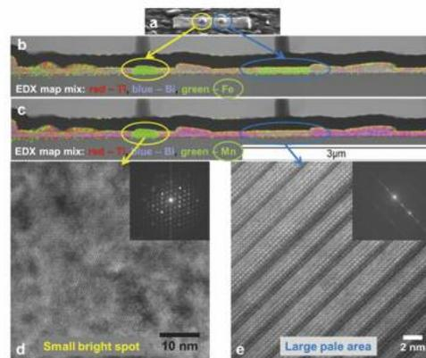
Some of the data presented in the paper published in Scientific Reports. The images depict the various points at which careful elemental analysis reveals the accumulation of some elements in specific regions of the deposited layer, together with evidence for the crystallinity and layer structure inherent to these materials.
