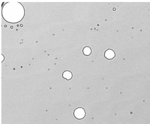
Acoustic image of bonded Si-to-Si wafer structure showing voided areas.
