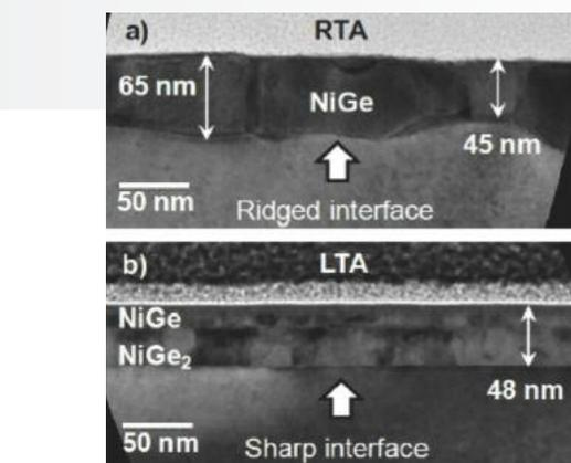
Representative Cross-Sectional Transmission Electron Microscopy Images of NiGe Layers Formed By (a) 350°C Rapid Thermal Anneal (RTA) and (b) Laser Thermal Anneal (LTA) With Energy Density of 0.45 J/CM<sup>2</sup>.
