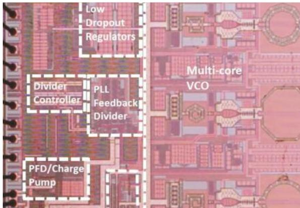
Micrograph of prototype synthesiser. The patented circuitry is labeled "Divider Controller".
