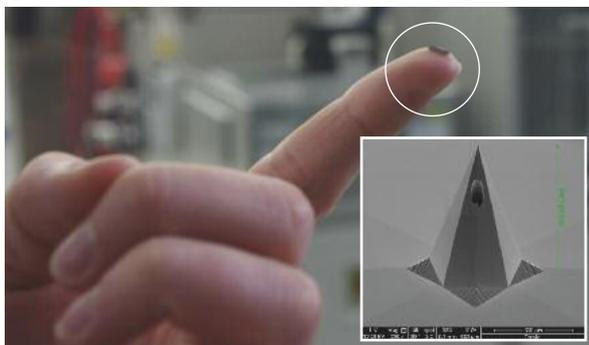
Hollow microneedles customised to deliver local anaesthetic during dental procedures.
