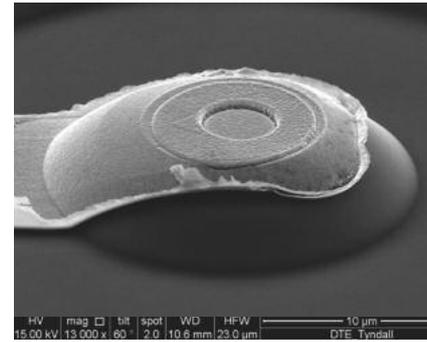
A single 16µm diameter DUV microLED.
