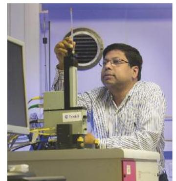
Dr Roy taking measurements in a SQUID Magnetometer.
