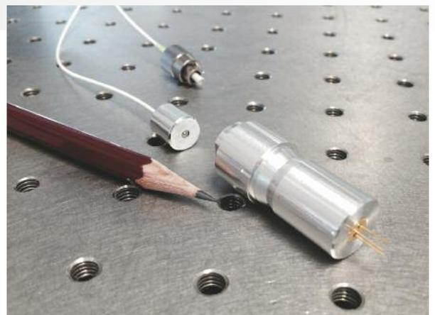
High power fiber-coupled laser module.
