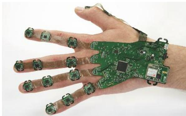
Wireless sensing glove enabling accurate measurements of hand and finger joint movement.
