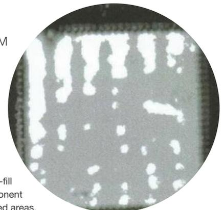
Acoustic image of under-fill quality in flip-chip component showing large voided areas.
